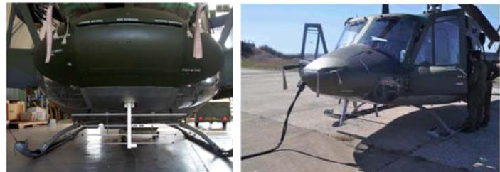
The deployed antenna is a log periodic one with four elements. This antenna has a 7dBi gain and a beam width of 68 degrees, with a front-back ratio of 15-19 dB. The antenna is mounted on a helicopter of the Italian Air Force and works as transmitter and receiver. The receiver acts with a minimum range gate delay of 4 μsec (for the measurement survey here presented a delay of 10 μsec was used) with a receiving time window of 81.5 μsec.
