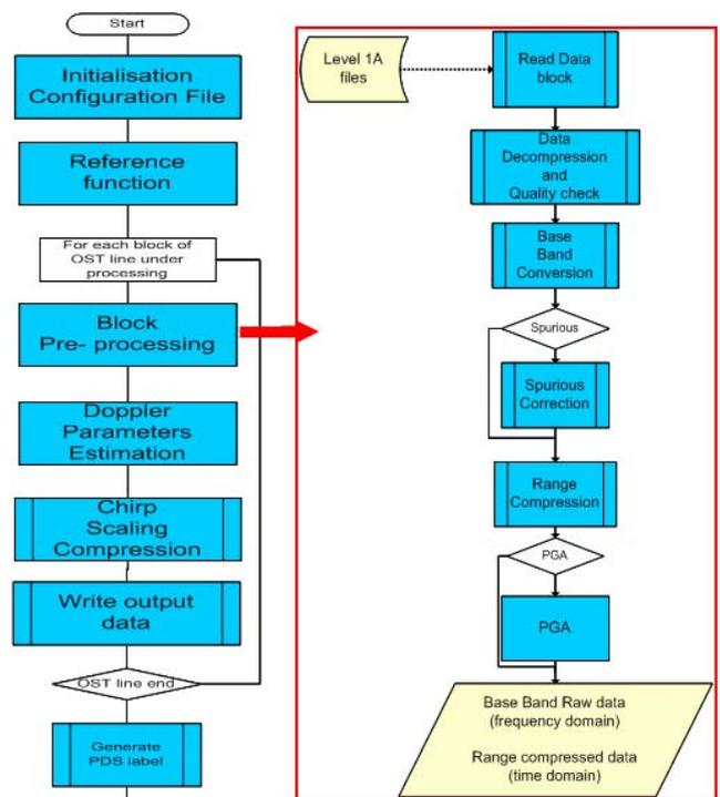
Figure 2. Flow Diagram of the ground processing applied on SHARAD data.
