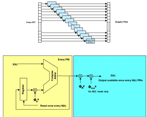
Figure 4 Azimuth Filter Structure
