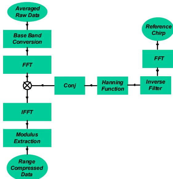
Figure 1 Block diagram of the range compression algorithm used for monitoring side-lobes.
