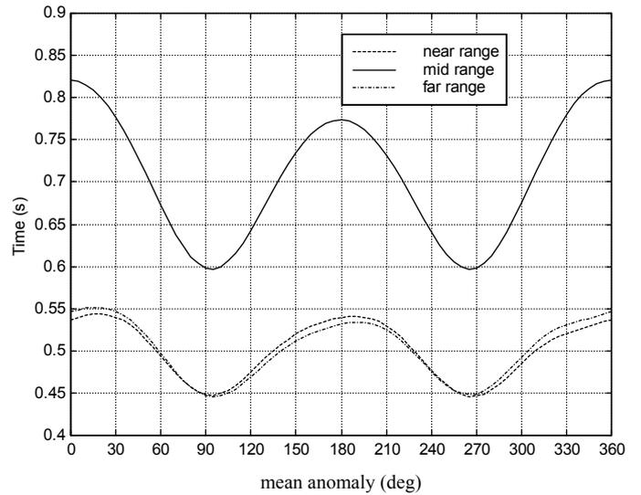
Fig. 4. Bistatic integration time as a function of BISSAT anomaly.
