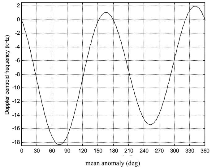
Fig. 1. Bistatic Doppler centroid frequency as a function of BISSAT anomaly.
