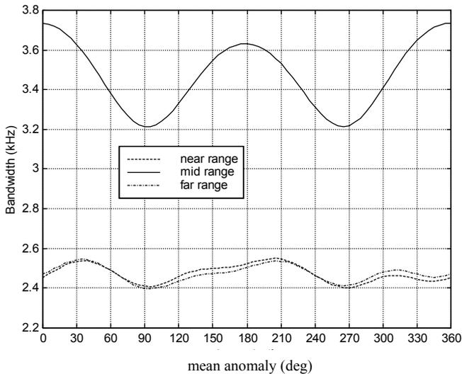
Fig. 3. Bistatic Doppler bandwidth as a function of BISSAT anomaly.
