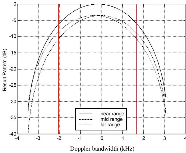
Fig. 2. Bistatic pattern along the azimuth aperture as a function of Doppler frequency at near, mid and far range (on the equator).
