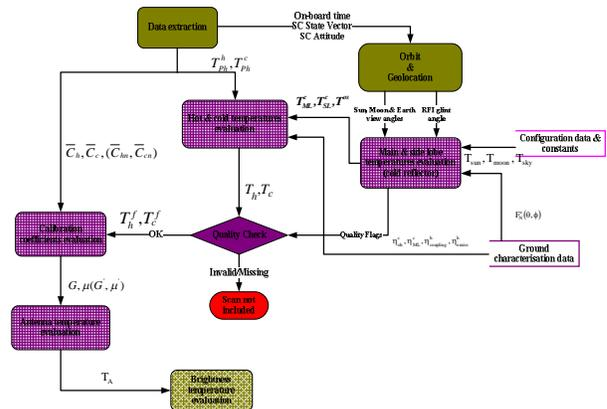
Figure 4: Flow diagram of radiometric calibration function (purple blocks) for MWI Level 1b processing chain.
