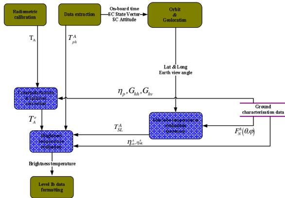
Figure 5: Flow diagram of brightness temperature function (blue blocks) for MWI Level 1b processing chain.
