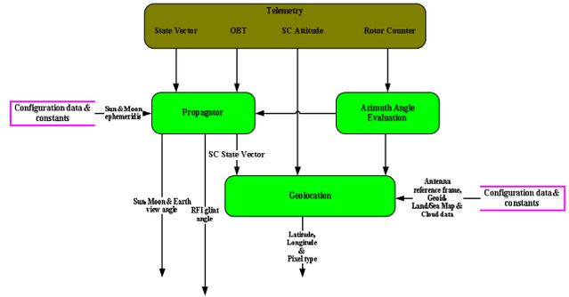
Figure 6: Flow diagram of orbit and geolocation function (high light green blocks) for MWI Level 1b processing chain.
