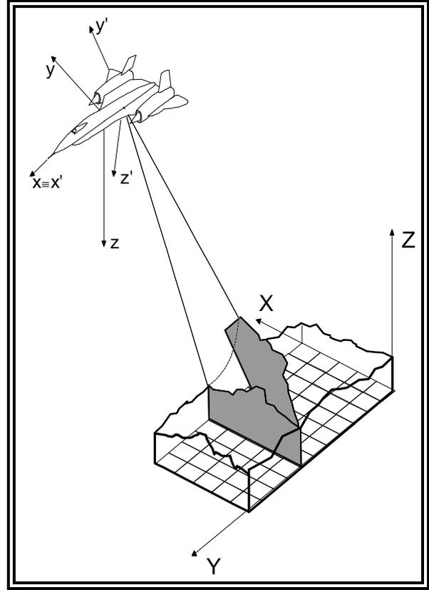
Figure 3. DEM projection geometry.
