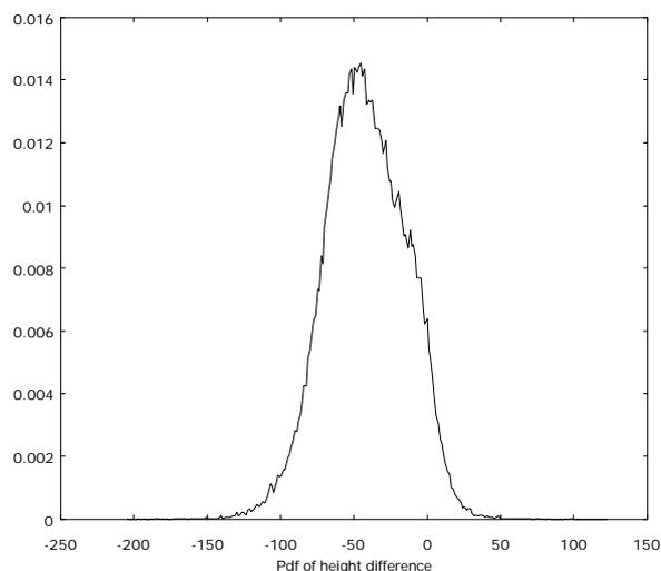
Figure 13. Interferometric DEM height error histogram.
