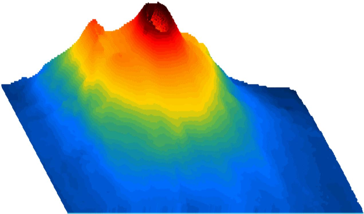
Figure 9. Three dimensional view of the interferometric DEM.
