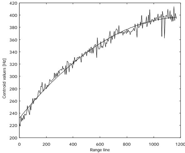
Figure 2. Estimated Doppler centroid variation along the swath and its least-square approximation.
