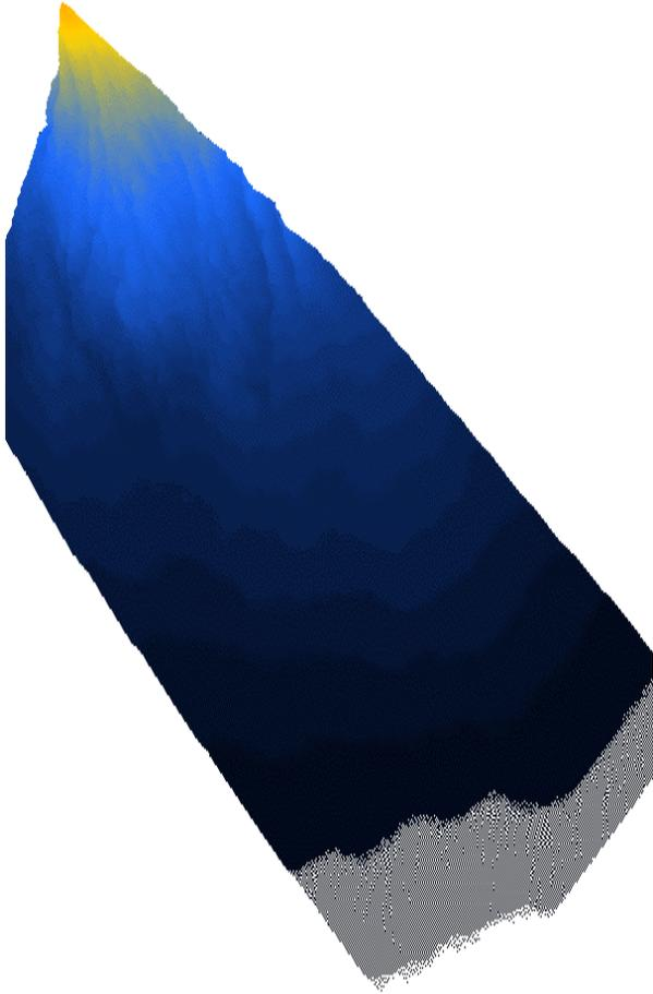
Figure 10. Slant range projection of the photogrammetric DEM: from azure (~50 m) to yellow (~1016 m).
