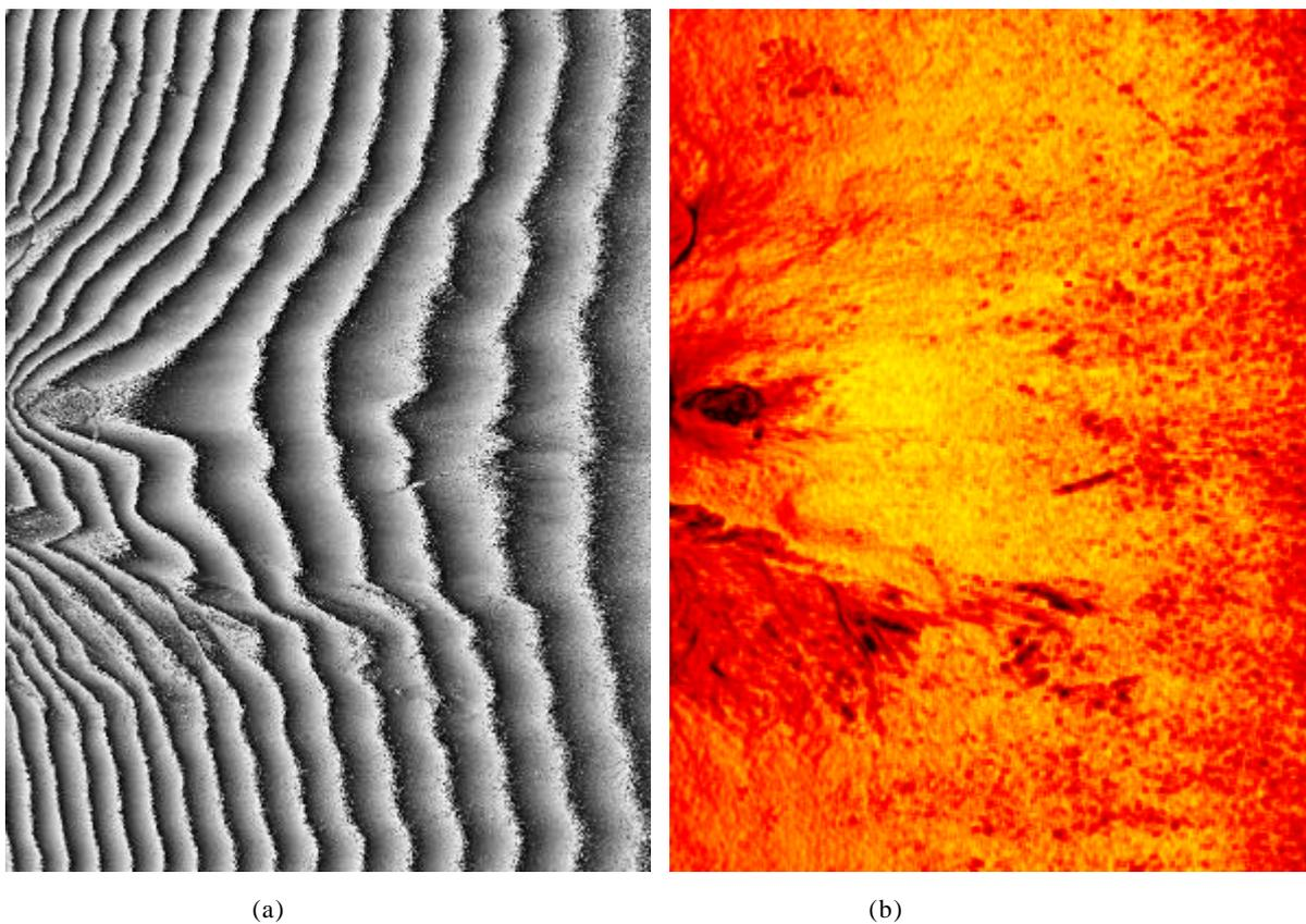
Figure 3. (a) Interferogram of the test-site; (b) Colour-coded coherence map, from black ( $|\gamma|=0.25$ ) to yellow ( $|\gamma|=0.85$ ).
