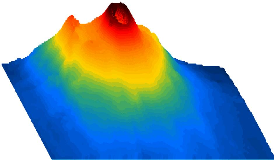
Figure 5. Colour-coded three-dimensional height map of Mt Vesuvius derived from the unwrapped interferogram.
