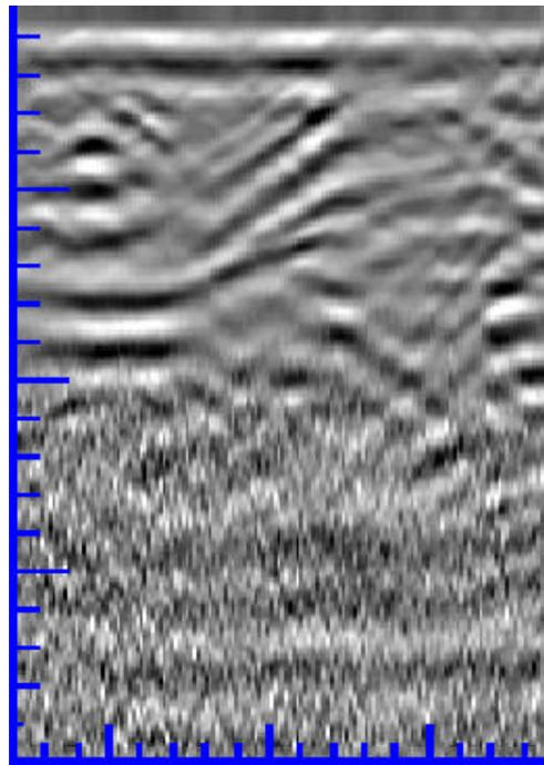
Figure 9: the two same pipes of figure 8 seen with a commercial GPR (courtesy of STRAGO s.r.l.)
