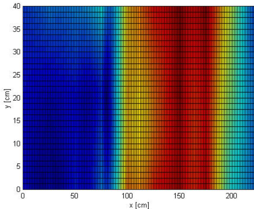
Figure 11: planar horizontal image of the metal sheet at 50 cm of depth corresponding to the return time of 15 ns
