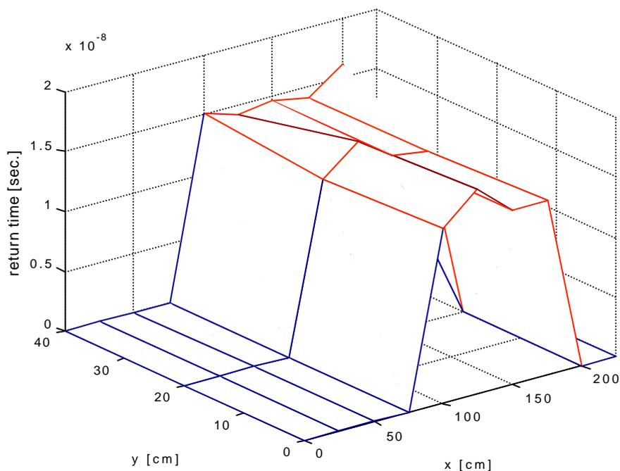
Figure 10: return times of the meaningful radar pulses on the metal sheet at 50 cm of depth (planar scan)
