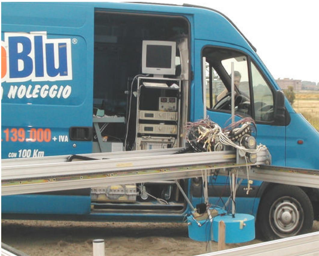
Figure 2: the rack of the GPR inside the van during data acquisition campaign
