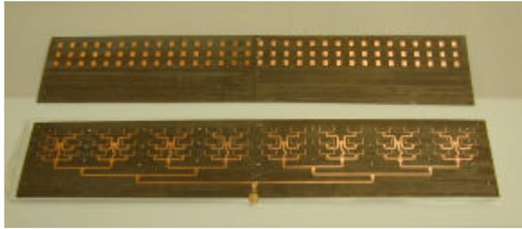
Fig. 3 – MiniSAR antenna prototype
