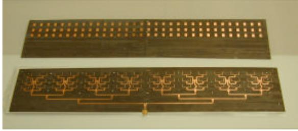
Fig. 3 – MiniSAR antenna prototype
