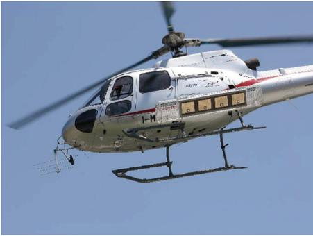
FIGURE 3: Sounder and imager antenna in flight configuration.
