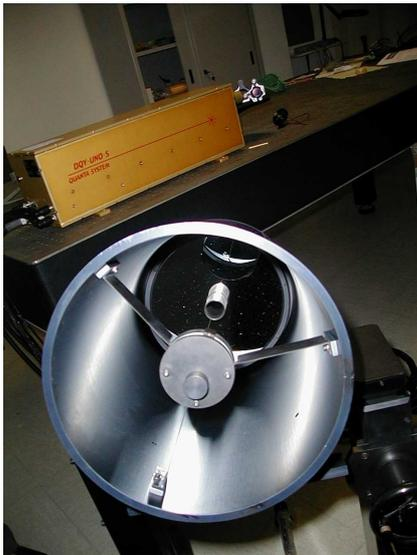
Fig. 4. A top view of the lidar Cassegrain telescope.
