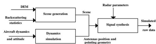
**Figure 1:** Block diagram of the SAR interferometer simulator
