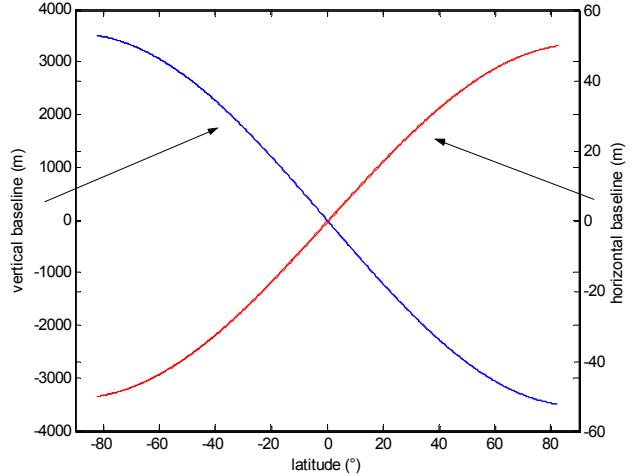
Figure 7 - Horizontal and Vertical Baseline as a Function of Latitude
