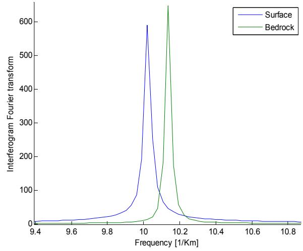
Figure 6 - Interferogram Fourier transform (By=50 m, Bz=3500 m, swath of 30 Km, bedrock depth of 3700 m)
