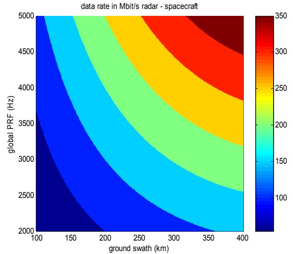
Figure 3 - Data rate from the radar to the spacecraft (single satellite)
