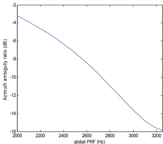
Figure 1 - Azimuth Ambiguity Ratio as a function of global PRF
