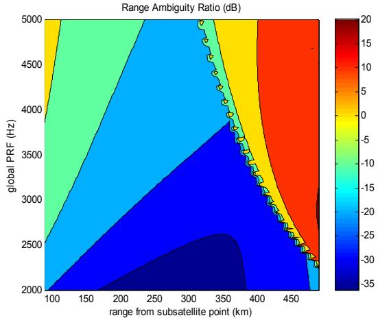
Figure 2 - Range Ambiguity Ratio as a function of global PRF and range from sub-satellite point
