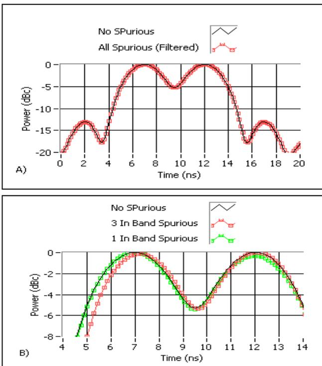
Figure 3. Simulation Results with new set of parameters: A) Simulated Targets without taking into account any spurious frequency (reference line) and by filtering all of them; B) Reference Line and 1 and 3 in band spurious signals.
