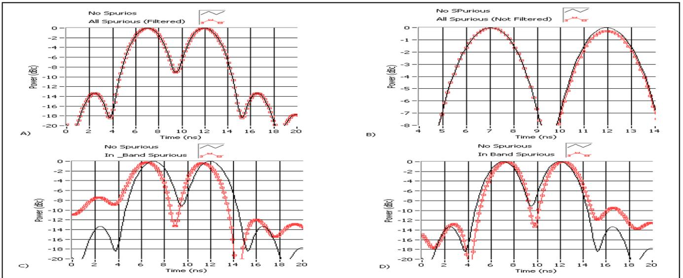
Figure 2. Simulation Results: A) Simulated Targets without taking into account any spurious frequency (reference line) and by filtering all of them; B) Reference Line and all out of band spurious frequencies without filtering; C) Reference Line and in band spurious frequencies ( $f_{s\_DDS}=1200$  MHz); D) Reference Line and in band spurious frequencies ( $f_{s\_DDS}=1100$  MHz)
