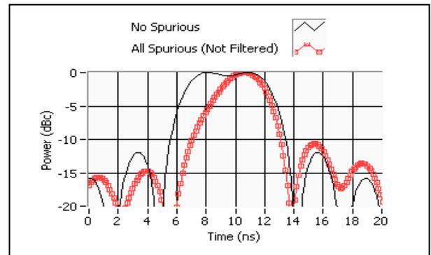
Figure 4. Simulation Results: Simulated Targets without taking into account any spurious frequency (reference line) and by not filtering all of them with two very close targets
