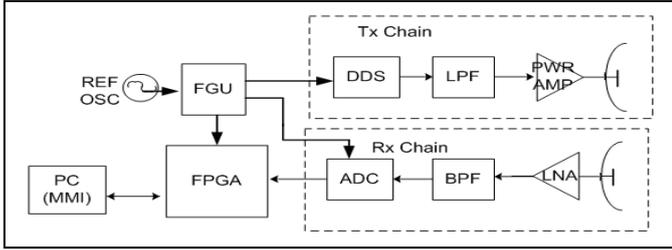
Figure 1. SFGPR architecture analysed in this paper.
