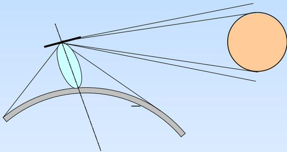
The effects of such radiation noise on SSR instrument can be evaluated by taking into account either the direct part coming from Jupiter and the portion backscattered by Ganymede's surface [1].
