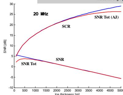
Final instrument performance can be evaluated by considering classical radar figure such as SNR (including Jovian radiation) and SCR. A model for signal ice attenuation is needed [4] as well as for ice temperature profile [5]
