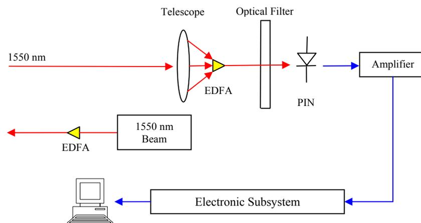
*Figure 11: Block diagram of the proposed Optical Ground Station*
