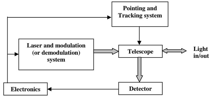
*Figure 1: High level block diagram of a terminal for optical satellite communication system*
