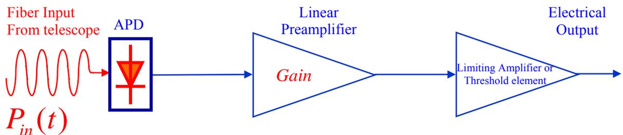
Figure 10: LEO Receiver block diagram
