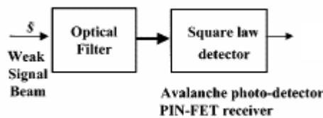
Figure 3: Direct detection receiver [1]
