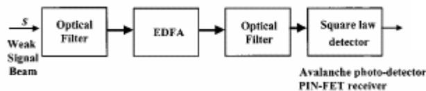
Figure 4: Pre-amplifier direct detection receiver (EDFA) [7]
