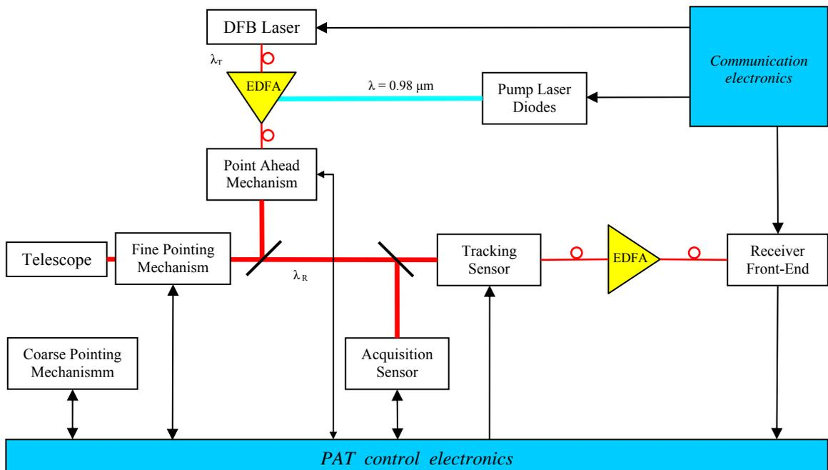
Figure 12: Optical terminal preliminary architecture of the OGS
