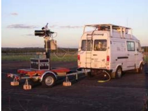
*Figure 7 : Mobile Ground Station of CAPANINA project (Communication from Aerial Platform Networks delivering Broadband Communications for All) [www.capanina.org]*
