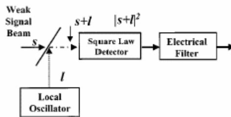
Figure 2: Coherent receiver [12]
