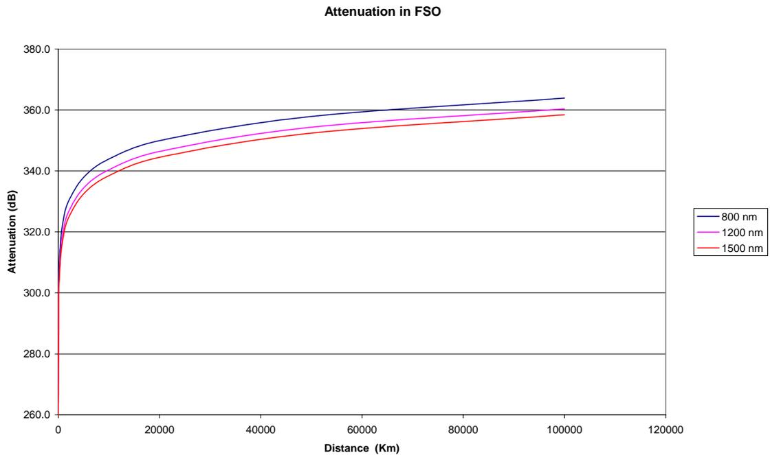
*Figure 8: Attenuation versus distances at different laser wavelengths*
