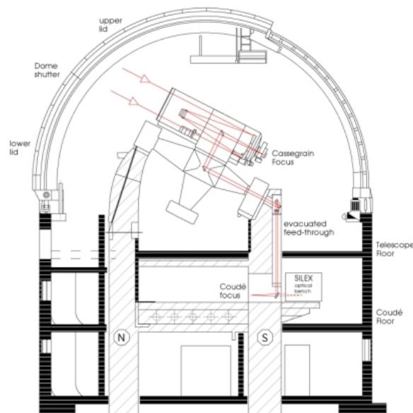
*Figure 15: Schematic layout of the OGS Telescope [26]*
