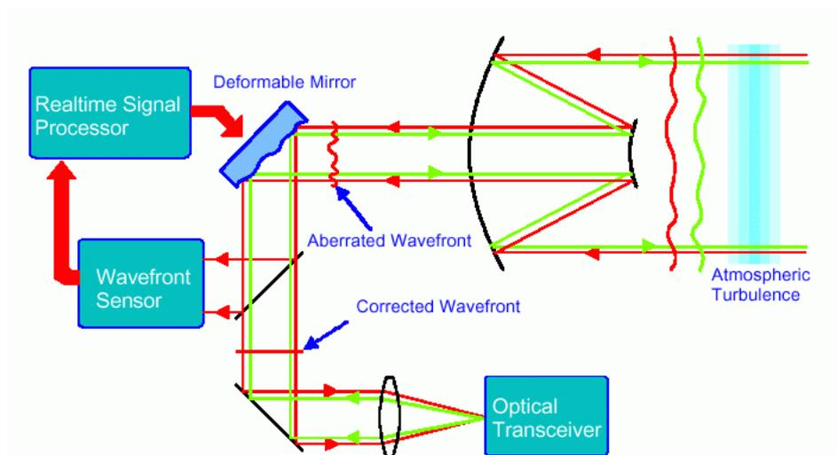
Figure 6: Schematic operation system of Adaptive Optics [[http://www2.nict.go.jp/mt/b162/ao\\_sys0-e.html](http://www2.nict.go.jp/mt/b162/ao_sys0-e.html)]
