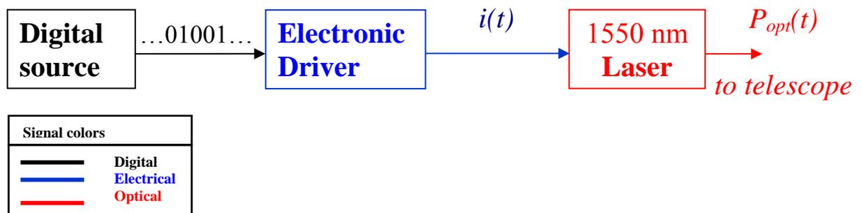
Figure 9: LEO Transmitter block diagram
