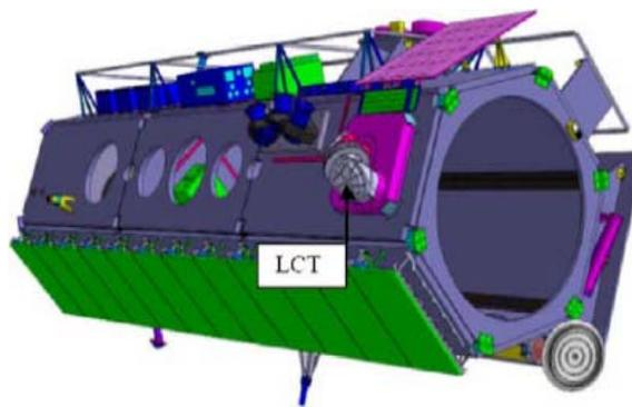
*Figure 22: Laser Communication Terminal (LCT) mounted on TerraSAR-X satellite, LCTSX [36]*
