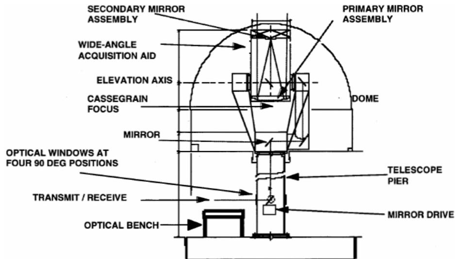
Figure 13: Schematic diagram of the Optical Ground Station [21]
