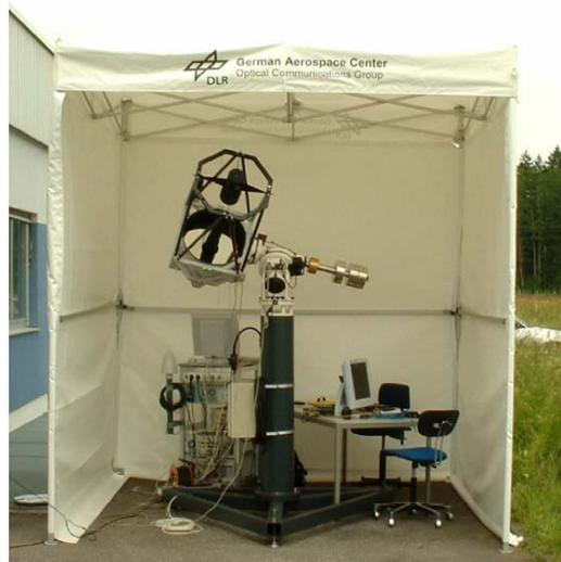
*Figure 23: Transportable Optical Ground Station during balloon trial in Kiruna, Sweden (August 2005) [37]*
