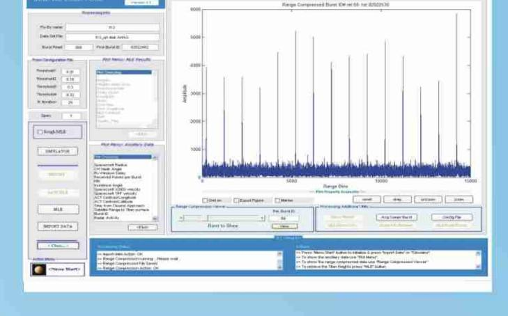
including procedures and algorithms designed to check and simulate the performances of the Cassini Radar Altimeter through calculation, visualization and plotting of relevant parameters (see Figure 5, showing an example of SLT GUI).
