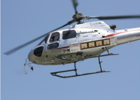
Figure 3. The sounder and imager antennas mounted on the civil helicopter.
