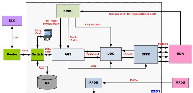
*Fig. 1 - ESS1 Architecture*
