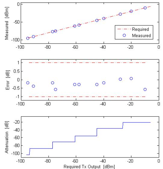
Fig. 5 - ESS1 Second Step Calibration Results
