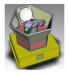
Figure 1: Conical scan microwave imaging radiometer layout
