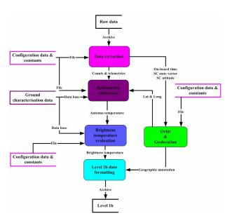
Figure 2: MWI/ICI architecture for Level 1b processing chain.
