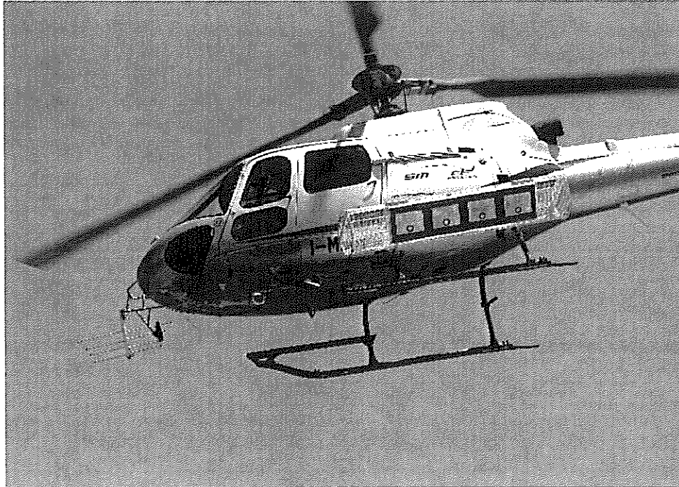
Fig. 1 - Photo of the sounder and imager antennas installed on the civil helicopter.
