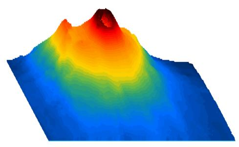
Figure 5. Colour-coded three-dimensional height map of Mt Vesuvius derived from the unwrapped interferogram.
