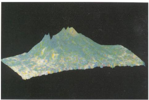
Figure 4. Three dimensional view of the interferometric DEM.
