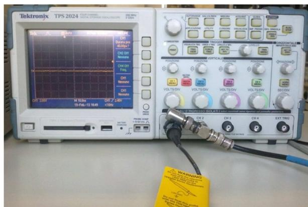
**Figura 126 - Tektronix TPS2024 a 4 canali 200MHz 2GS/s**
